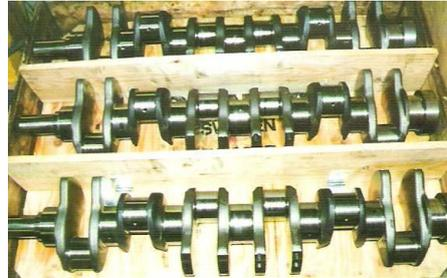
250 Crankshafts under machined by 100 Microns saved by Selective Plating.
